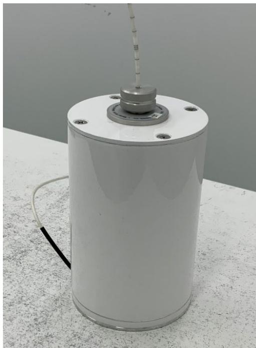
**Figure 1.** Well type chamber used for brachytherapy calibration
