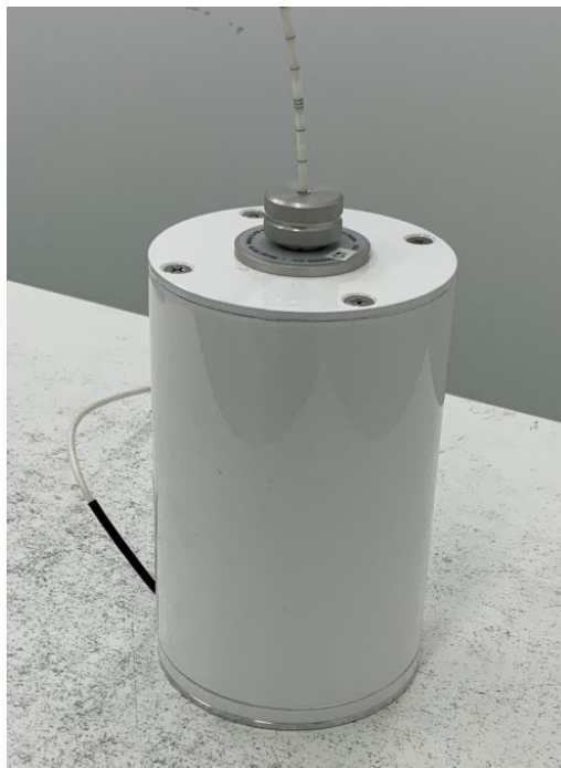
Figure 1. Well type chamber used for brachytherapy calibration
