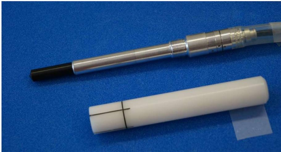
**Figure 1.** Transfer chamber type FC65-G
