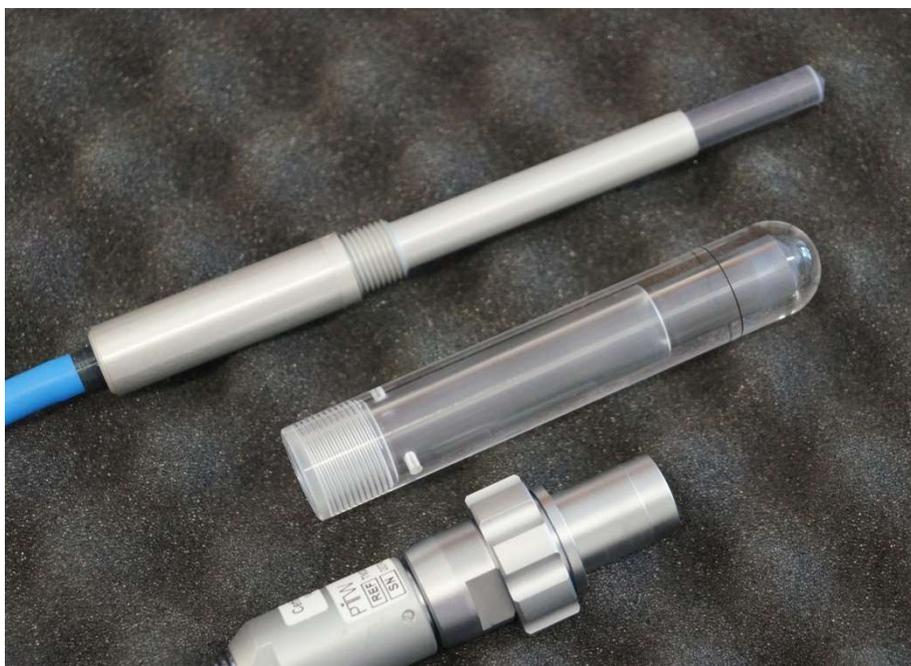
**Figure 2.** Transfer chamber type PTW 30013
