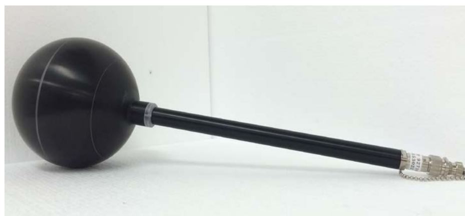
Figure 1. Transfer chamber type Exradin A6
