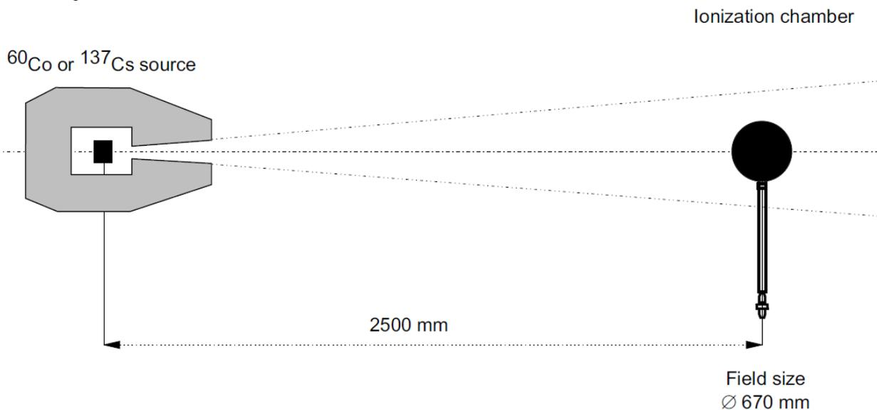
FIG. 2. Set-up for calibration in terms of air kerma for  $^{137}\text{Cs}$  and  $^{60}\text{Co}$  gamma beams.
