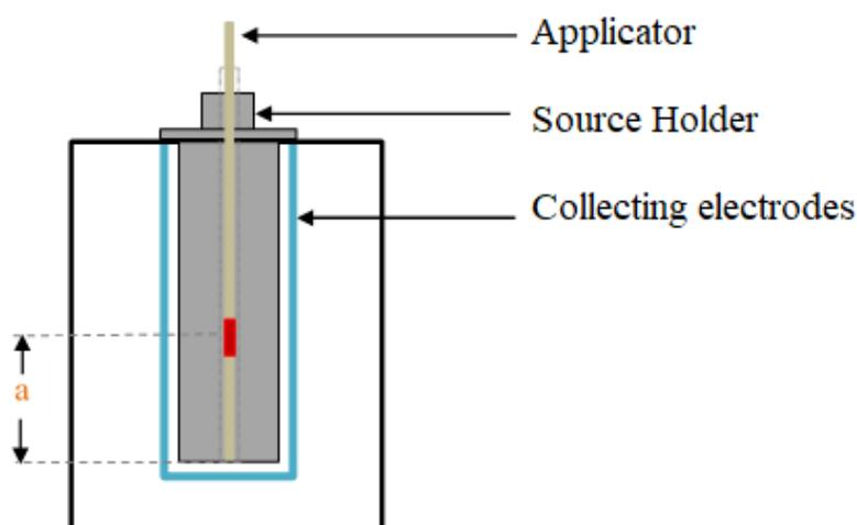
**Figure 1:** Measurement setup for the calibration of the well-type chamber using HDRBT sources. The height “a” is the point of maximum response of a well-type ionization chamber “sweet spot”.
