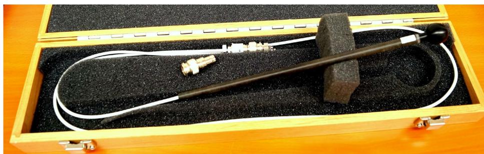
**Figure 1.** Transfer chamber type Exradin A3
