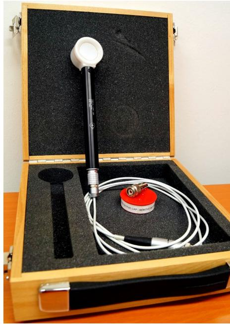
**Figure 2.** Transfer chamber type Radcal RC6M
