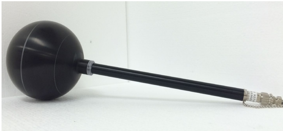
Figure 1. Transfer chamber type Exradin A6
