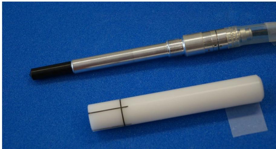
**Figure 1.** Transfer chamber type FC65-G
