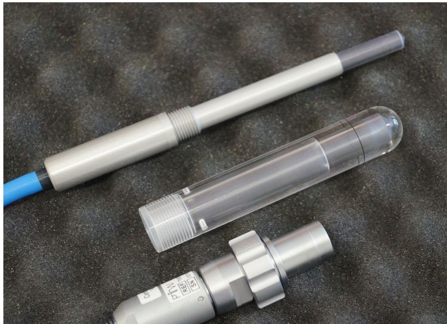
**Figure 2.** Transfer chamber type PTW 30013
